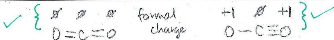
Left hand structure is the most stable as the atoms have no formal charges. ✓
