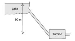
The mass flow rate of the water is  $3000 \text{ kg min}^{-1}$ . The turbine has an efficiency of 60%. Acceleration due to free fall is 10 m s<sup>-2</sup>.
