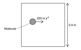
Assume all collisions between the molecule and the walls of the container are perfectly elastic.
