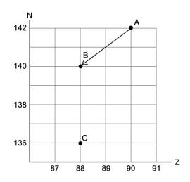
Three more decays occur before  ${}^{224}_{88}\it{Ra}$  is produced, denoted by "C" on the N-Z diagram.
