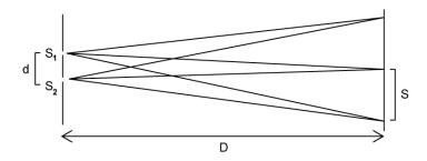
The separation distance of the slits d = 0.2 mm, and the distance between the slits and the screen D = 1.2 m.
