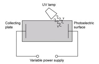
The photoelectric surface is grounded, and the variable power supply is adjusted so that the electric potential of the collecting surface is 1.5 V.
