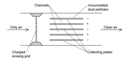
A dust particle of mass  $6.7 \times 10^{-15}$  kg enters the region between the collecting plates travelling horizontally with an initial velocity of 11 m s<sup>-1</sup>. The particle carries a charge of  $2.6 \times 10^{-18}$  C.
