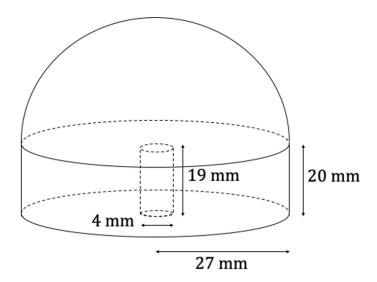
(a) Show that the volume of material required to construct the doorknob is  $27626\pi$  mm<sup>3</sup>.
