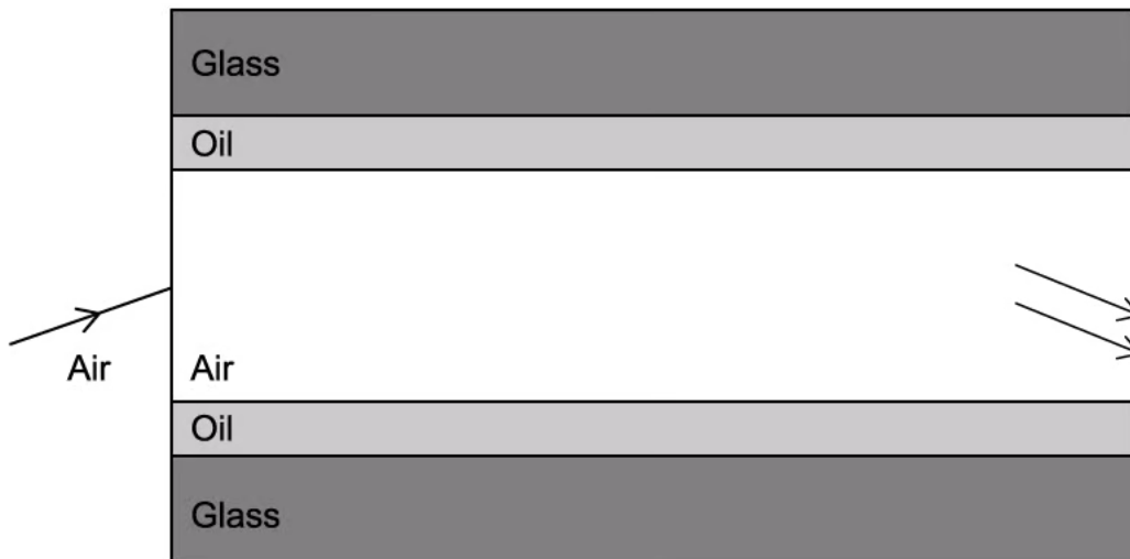
Damaged optical fibre
