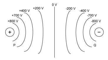
The electric field strength Evaries along the line which connects P and Q.
