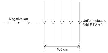
It enters a uniform vertical electric field of strength  $V\,kV\,m^{-1}$ , which is directed downwards and acts over a horizontal distance of 100 cm.
