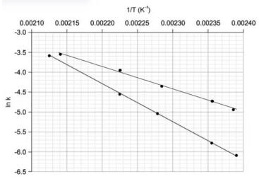
State which plot shows the reaction with the greatest activation energy.
