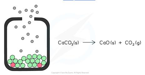
The diagram shows an open system in which the calcium carbonate is continually decomposing as the carbon dioxide is lost causing the reaction to eventually go to completion
