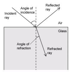
The angle of incidence is less than that of the critical angle. The refractive index of the glass is 1.50.
