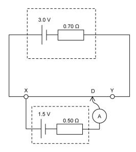
The moveable contact can again be connected to any point along the wire XY. At point D, there is zero current in the ammeter.
