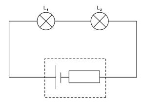
The lamp  $L_1$  has a resistance of 10  $\Omega$  and  $L_2$  has a resistance of 25  $\Omega$ .
