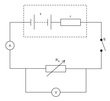
A variable resistor, which acts as the load resistance  $R_L$ , is connected to a power source of e.m.f.  $\varepsilon$  and internal resistance r, along with a switch S and an ammeter and voltmeter.
