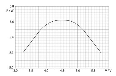
(a) Assuming the Maximum Power Theorem is valid, use the graph to determine the internal resistance of the power source.
