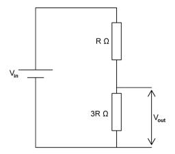
$$A. V_{out} = \frac{1}{4} V_{in}$$
