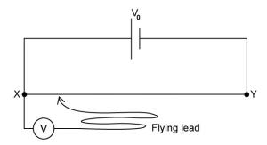
The flying lead connected at X and is able to connect to XY at any distance r from X.
