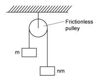
What is the acceleration of the masses a and the tension in the string T?
