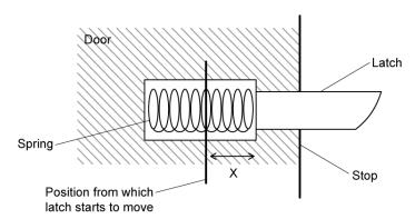
When the latch is pushed in, the spring compresses.
