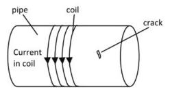
Cracks along or parallel to the length of the pipe do not show up.
