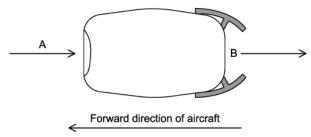
In one second a mass of  $3.75 \times 10^5$  g of air enters A and the speed of this mass of air increases by 587 m s<sup>-1</sup> as it passes through the engine.
