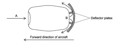
The speed of the deflected air is the same as the speed of the air leaving B.
