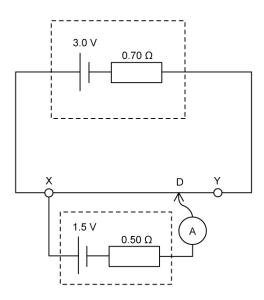
$The moveable \ contact \ can \ again \ be \ connected \ to \ any \ point \ along \ the \ wire \ XY. \ At \ point \ D, \ there \ is \ zero \ current \ in \ the \ ammeter.$
