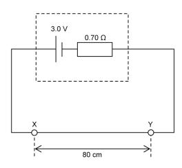
The resistivity of the metal used to make the wire is  $1.10 \times 10^{-6} \Omega$  m.
