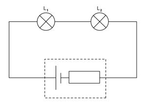
The lamp L<sub>1</sub> has a resistance of 10  $\Omega$  and L<sub>2</sub> has a resistance of 25  $\Omega$ .
