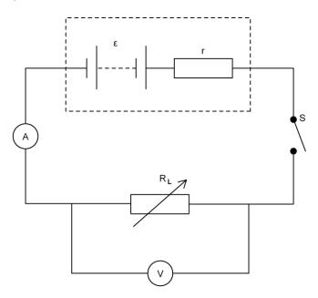
A variable resistor, which acts as the load resistance  $R_L$ , is connected to a power source of e.m.f.  $\varepsilon$  and internal resistance r, along with a switch S and an ammeter and voltmeter.
