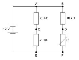
The battery has an e.m.f. of 12 V, with negligible internal resistance. At room temperature, the resistance of the thermistor is  $4.0 \text{ k}\Omega$ .
