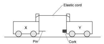
The two trolleys are pulled apart so that the elastic cord is stretched. The trolleys are then released at the same time and move towards each other. The trolleys stick together on impact.
