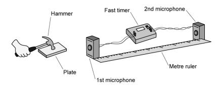
The microphones were placed 80 cm apart. The mean time interval was 2.5 ms.
