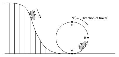
As the passengers move around the circle from  ${\bf A}$  to  ${\bf B}$  to  ${\bf C}$ , the reaction force between exerted by their seat varies.
