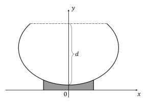
The glass part of the bowl sits on a solid base, indicated by the shaded region on the diagram. The cross-section of the glass part of the bowl is symmetrical about the *y*-axis, and may be described by the curve with equation
