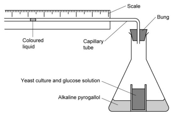
When the researcher inserted the bung and began the experiment, the coloured liquid initially moved to the right. After a period of time, the coloured liquid slowed, stopped and reversed its direction, moving to the left.
