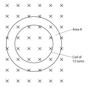
What is the magnetic flux linkage for the coil?
