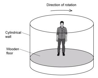
The fairground ride is then rotated. When the ride is rotating sufficiently quickly the wooden floor is lowered. The riders remain pinned to the wall by the effects of the motion. When the speed of rotation is reduced, the riders slide down the wall and land on the floor.
