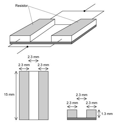
The material from which each resistor is made has a resistivity of  $2.0 \times 10^5 \,\Omega$  m and both resistors have dimensions of 15 mm by  $2.3 \,\mathrm{mm}$  by  $1.3 \,\mathrm{mm}$ .
