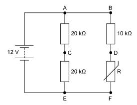
The battery has an e.m.f. of 12 V, with negligible internal resistance. At room temperature, the resistance of the thermistor is  $4.0 \, k\Omega$ .
