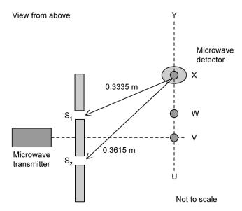
The microwaves from the transmitter are polarised. These waves are detected by the aerial in the microwave detector (probe). The aerial is a vertical metal rod.
