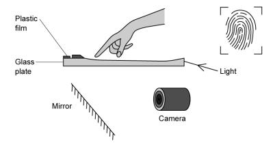
When not in use, the plastic screen and the glass have a small air space between them. The diagram below shows the two possible paths for the light when the finger is pressed down.
