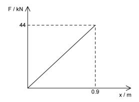
(d) Using the area under the graph, show that the spring constant of the spring is about  $49 \, \text{kN m}^{-1}$ .
