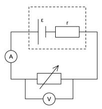
The student wishes to determine the relationship between the voltmeter and ammeter readings whilst decreasing R. Their results are given.
