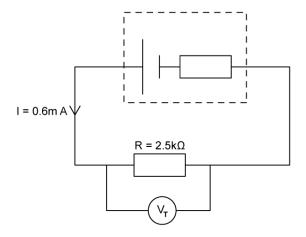
(c)  $\label{eq:calculate} \mbox{Calculate the terminal potential difference $V_T$ of the circuit.}$
