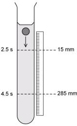
There are two marks on the tube. The top mark is positioned at  $15 \pm 1$  mm on the adjacent rule and the lower mark at  $285 \pm 1$  mm. The ball passes the top mark at  $2.50 \pm 0.02$  s and passes the lower mark at  $4.50 \pm 0.02$  s.
