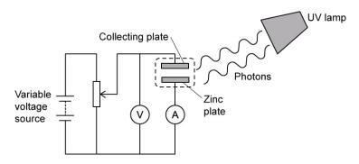
Photoelectrons are emitted from the zinc plate and move towards the positive collecting plate due to the potential difference, *V*, between the plates. When the potential difference, *V*, is varied, it is observed that the photoelectric current varies as shown on the graph.
