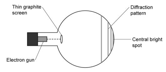
A pattern forms when diffracted electrons are incident on a fluorescent layer at the end of the tube.
