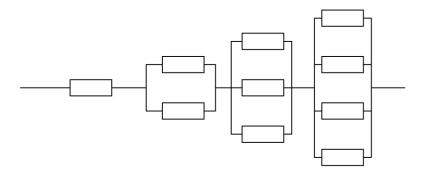
(a) Show, without the use of a calculator, how to find the value of resistance of each resistor and hence determine the value of R.
