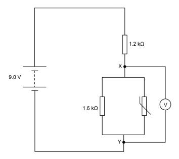
Show, without the use of a calculator, how to determine the reading on the voltmeter, giving the answer to two significant figures.
