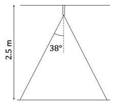
(a) Calculate the horizontal distance on the floor that is illuminated by the lamp.
