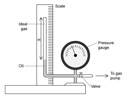
The pump forces the oil to move up the tube and so reduces the volume of the gas. The scientist measures the pressure p of the gas and the height H of the column of gas.
