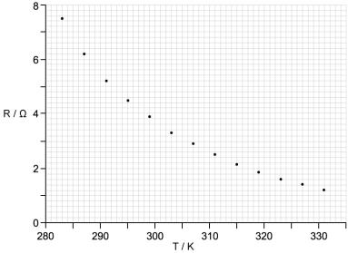
The electric current through the thermistor for  $T = 283 \, \text{K}$  is  $0.0078 \, \text{mA}$ .
