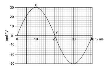
The resistance of the coil is 10.0  $\Omega$ . Which of the following values gives the average power dissipated in the loop?
