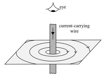
(ii) current in one turn produces magnetic field in region of adjacent turn; this gives rise to force in adjacent turn which also has electric current; they attract;
