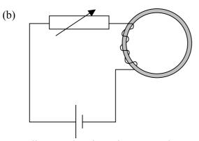
diagram showing wire wrapped around part of the ring;<br/>and appropriate connections to battery and variable resistor;<br/>as the current is changed by altering the value of the resistance;<br/>a current is induced in the ring;[4]Mark diagram and description together – look for any sensible description of the<br/>production of transformer induced currents.[4]
