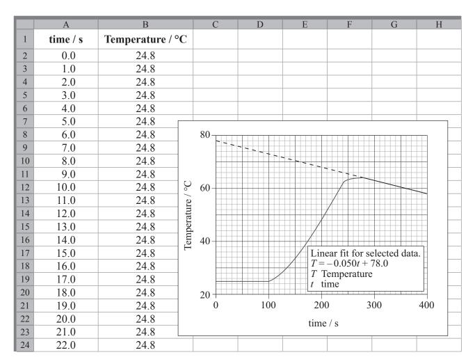
A straight line has been drawn through some of the data points. The equation for this line is given by the data logging software as
