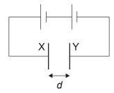
The capacitor has a capacitance *C* and a charge *Q*. The plates X and Y of the capacitor are a distance *d* apart. Edge effects are negligible.
