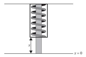
The displacement, x, of the spring is measured, in centimetres, from the equilibrium position of x = 0. The value of x can be modelled by the following second order differential equation, where t is the time, measured in seconds, after the initial displacement.
