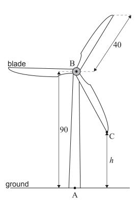
The end of one of the blades of the turbine is represented by point C on the diagram. Let h be the height of C above the ground, measured in metres, where h varies as the blade rotates.
