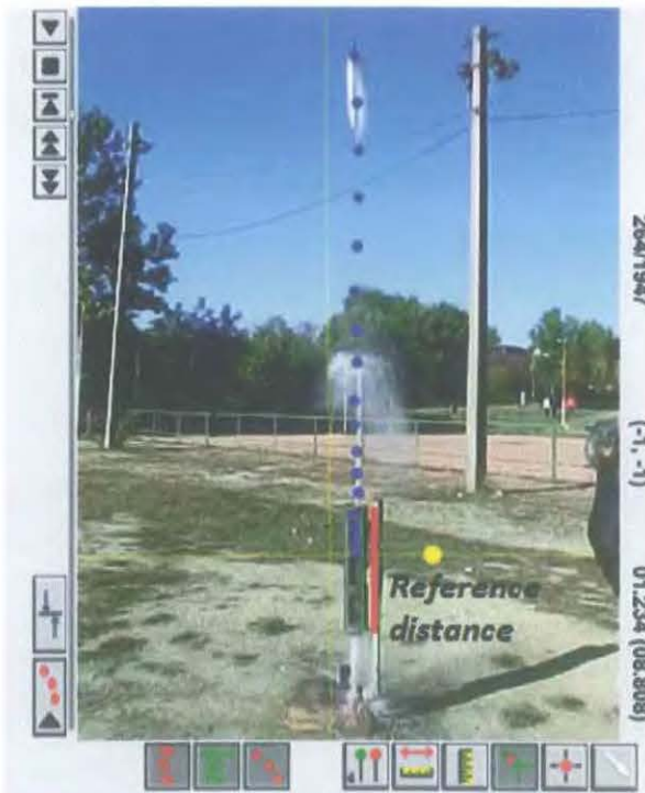
Figure 10: The method of examining every second frame in Logger Pro 3.8.4. The red line is a reference distance which is 0.58 m.
