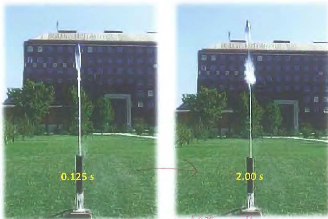
Figure 8: A water rocket, just after it ejected all of its water
