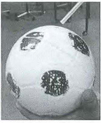
Figure 3 This photo shows air being blown across the hole in the ball. Note that the angle, the distance from the ball, and power of the air coming from the straw should be constant for each trial of a certain ball.
