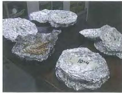
Figure 5. The wheat being packed inside the aluminum foil, in order to be put in the oven.
