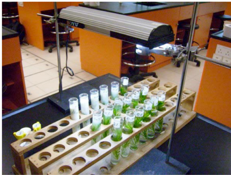
Figure 10: Experimental setup for test on phytotoxicity of Insecticide on Elodea canadensis
