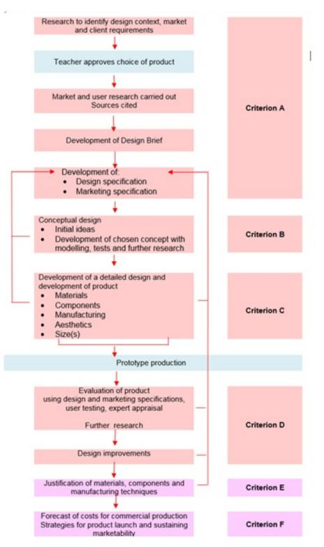
Figure 1: An example of an iterative approach to the Design Project
